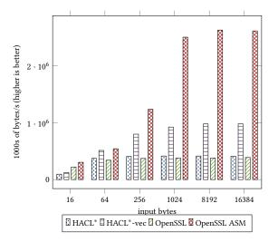
Figure 10: OpenSSL speed comparison for the Chacha20 algorithm. The algorithm is run repeatedly for three seconds on different input sizes, and we measure the number of operations via the openssl speed command. The experiment is performed on an Intel Core i7 @ 2.2Ghz running OSX 10.12.4.
