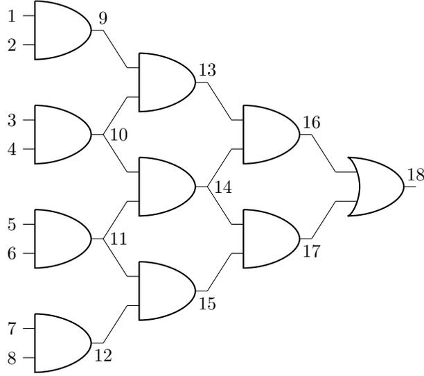
Figure 2: Circuit with consecutive layers of AND gates
