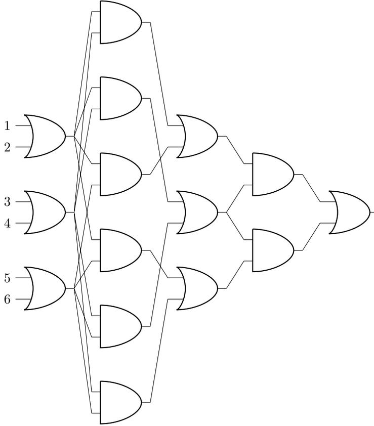
Figure 4: Circuit in Figure ?? blown-up to apply the Free-OR technique
