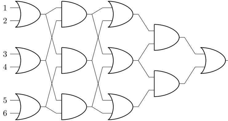
Figure 3: Circuit illustrating use of the Free-OR technique
