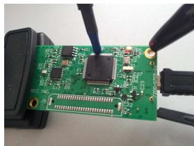
(b) LF-B-3 positioned near the VCC pin.
