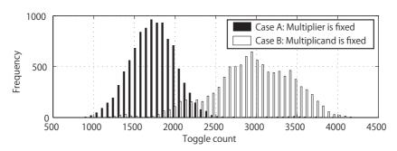
Fig. 3. Toggle counts of a 32-bit multiplier
