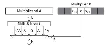
Fig. 2. A circuit for generating a partial product in the radix-4 Booth recoding
