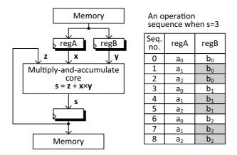
Fig. 4. A common circuit architecture for LIM
