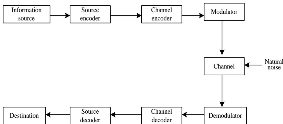
Figure 1: A typical transmission system aims at communication reliability
