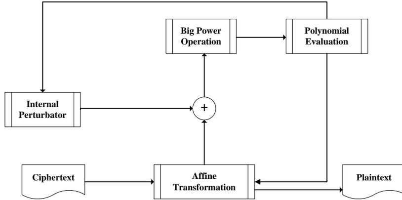
**Fig. 2.** The hardware structure of PMI+ Decryption
