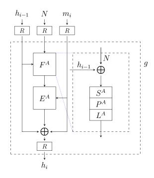
Figure 8: The Modified Compression Function for AES-like Representation
