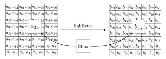
Figure 4: The S (SubBytes) Transformation
