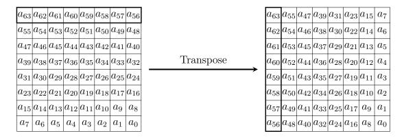
Figure 5: The P (Transposition) Transformation
