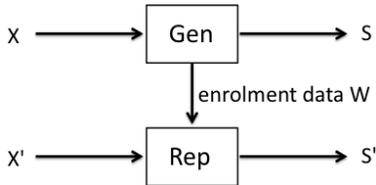
Figure 1: *Fuzzy Extractor*. **Gen** generates public data  $P$  and a near-uniform key  $S$ . **Rep** tries to reproduce  $S$  from  $P$  and a noisy measurement  $X'$ .
