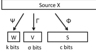
Figure 2: The AUHF's  $\Psi_t$ ,  $\Gamma_j$  and  $\Phi_r$  compresses  $X$  to  $k$ ,  $\sigma$  and  $c$  bits, respectively. The concatenation  $\Psi\Gamma\Phi$  is also an AUHF.
