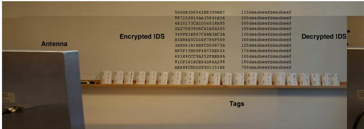
Figure 4: **Implementation setup and results** An example implementation setup shows an RFID reader and antenna, 20 TSS-encoded tags, and two screenshots depicting example encrypted and decrypted reads.
