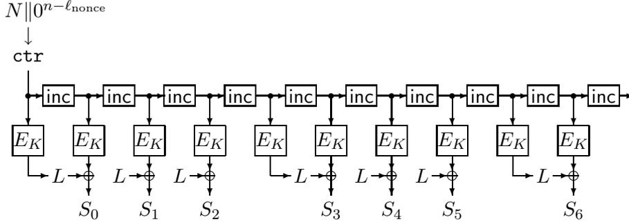
Figure 3: Illustration of the keystream generation algorithm. This example uses  $w = 3$  and outputs  $l = 7$  blocks of keystream  $S = (S_0, \dots, S_6)$ . This  $S$  is used in both encryption and decryption. The mask  $L$  is updated after generating  $w$  blocks of keystream. The counter  $ctr$  is incremented for  $l + \lceil l/w \rceil = 10$  times, and there are 10 blockcipher invocations.
