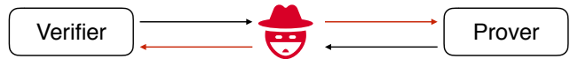
Fig. 2. In Mafia Fraud, an external attacker reduces the distance measured between two mutually trusted parties.
