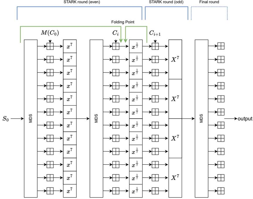
Figure 3: One round of the XHash8 permutation
