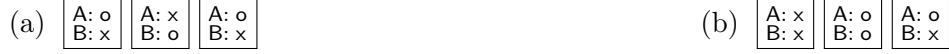
Figure 2: Two ways of voting for the second candidate (candidate B) in the ThreeBallot protocol, where x represents a marked position and o represents an unmarked position. All the other possibilities of voting for B can be obtained as permutations of these two.
